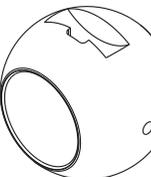
19. Locate the body on center line of pipe work, fit body connector bolts and nuts.
